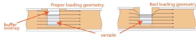
1. **Re-check the buffer level in the sample wells.** Make sure that sample wells are completely full to the top with electrophoresis buffer. Fill with additional buffer, if necessary.
