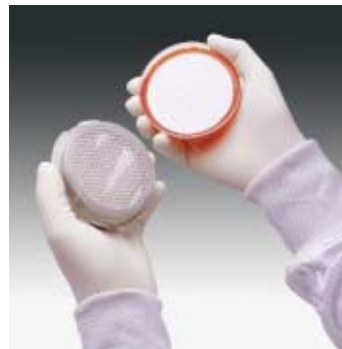
Direct Transfer Method Direct transfer of gelatin membrane to agar plate for fast, accurate detection of microorganisms.
