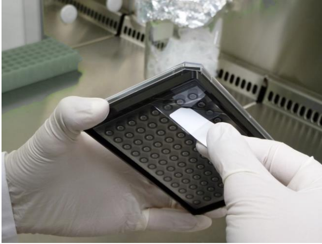
Fig.4: Pull off the protection foil.
