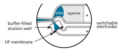
Users enter a target value or size range in software, and the selected DNA fragments are collected in buffer. Collections are removed with a standard pipette.
