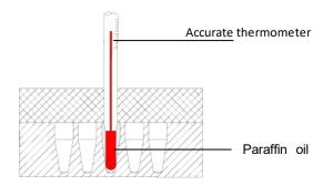
3) Press button and of Temp to start calibrate. Time window displays "Adjt", temperature displays the instant temperature of block with dot flickering, and instrument starts to heat up to 40.0°C.
