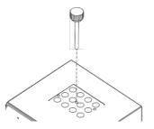
7.3 Lift upward the block lifter and take out block.
