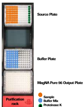
Figure 3: Purification rack loading schema for cfNA 2000 protocols.
